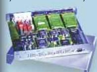
data stream, rather than paying high costs for the one expensive large physical channel to send this data, the Imux can break it down into small pieces and send them over smaller, cheaper separate physical channels.
