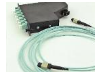
(MPO) An MPO cable with a breakout cassette from MPO to 12 x LC connectors
