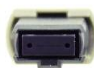
(MPO Connector close picture) The above picture shows the end of a 12 core fibre lead. The two big pins at either side are the precision locating pins. The 12 fibre cores can be seen across the centre of the connector between the locating pins.
